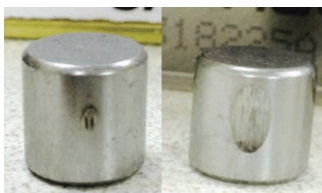
A smooth metal test piece installed on a lever, a hardened metal turning wheel immersed in sample oil driven by electric motor. While turning oil is driven up between rubbing surface of wheel. By adding weights to lever on left causing load/pressure between test piece and turning wheel. PPE Nano n Lubricants hold up more than 30 weights while wheel continues to turn and causing very little wear.
