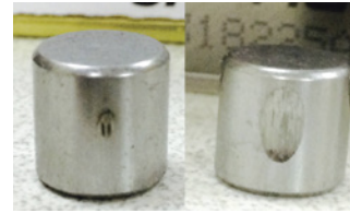
Right Same Timken experiment is performed on metal piece after engine oil after six-month and 15,000km of service. (2010 Honda Civic 1.8, Extreme 0W-30 is being tested)
